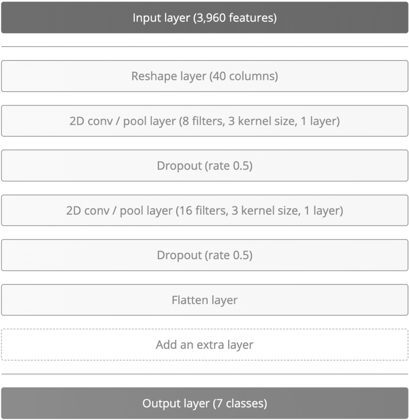
Figure 4.30: Expected CNN architecture in visual mode
